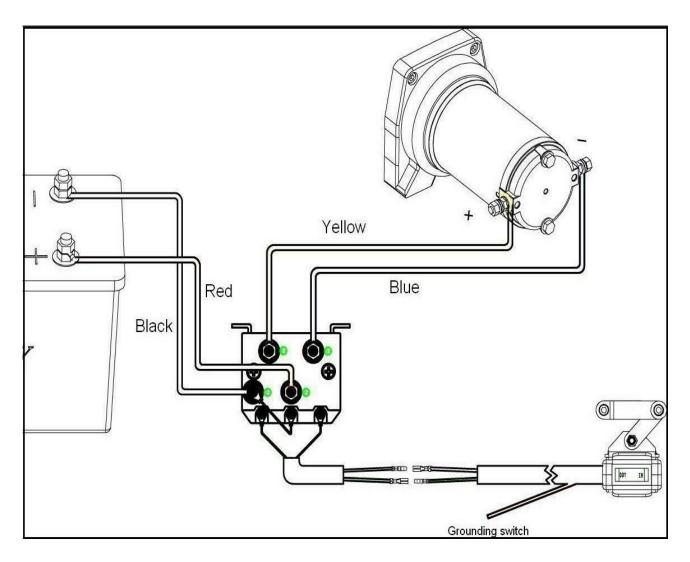
Figure 7 Wiring instalation diagtam
