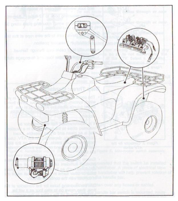
Figure 1: To install the complete kit, you will need to mount the winch, contactor handlecar mounted Mini-rocker switch. Mounting locations may vary depending on make and model of the ATV. Read and understand the following instructions to choose the appropriate mounting locations.
