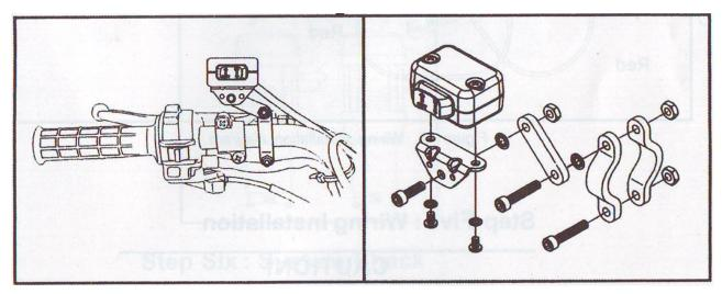
Figure 4: handlebar mount, Exact positioning may vary decending on ATV make and model.
